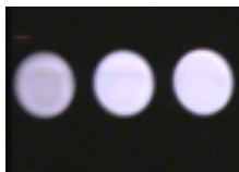
Figure 4-2 - Reference phantom of ICG solution- from left to right; 5.0, 10, 25 \mu\text{M} /ml
