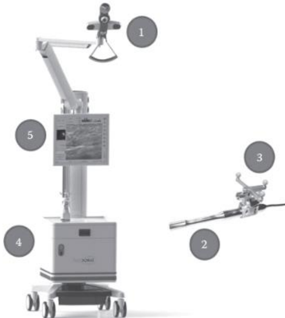
Figure 2-4 - Components of freehand single-photon emission computed tomography device (fhSPECT), declipseSPECT, image provided by SurgicEye GmbH, Germany.
