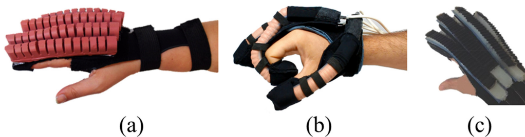
Figure 61 – Elastomer-based soft exoskeleton systems for the hand: (a) the system developed by the research team from Harvard (Cambridge, MA, USA) based on PneuNets [290], (b) a development of the same system reinforced with fabric sleeves [34], (c) the MRC-Glove, an MRI compatible solution developed by the research team from the National University of Singapore (Singapore) [289].
