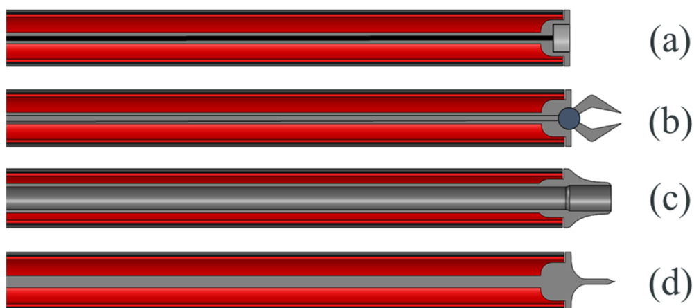
Figure 53 – Possible implementation of the Inflatable Arm as flexible laparoscopic tool: (a) endoscope, (b) gripper or cutter, (c) aspirator/irrigator, (d) RF ablation tool.
