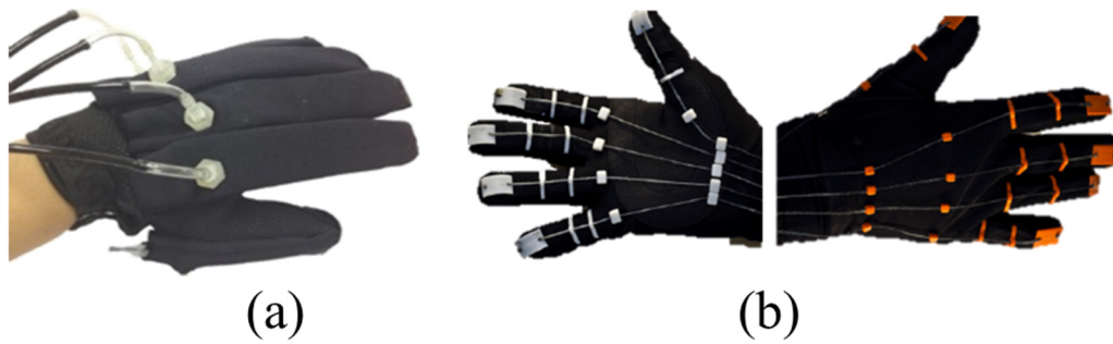
Figure 62 – Fabric-based soft exoskeleton systems for the hand: (a) a fluidically actuated system using flexible plastic actuators embedded in fabric pouches developed by the research team from the National University of Singapore (Singapore) [295]; (b) the palm and the back side of the tendon-driven system developed by the research team from the Worcester Polytechnic Institute (Worcester, MA, USA) [291].
