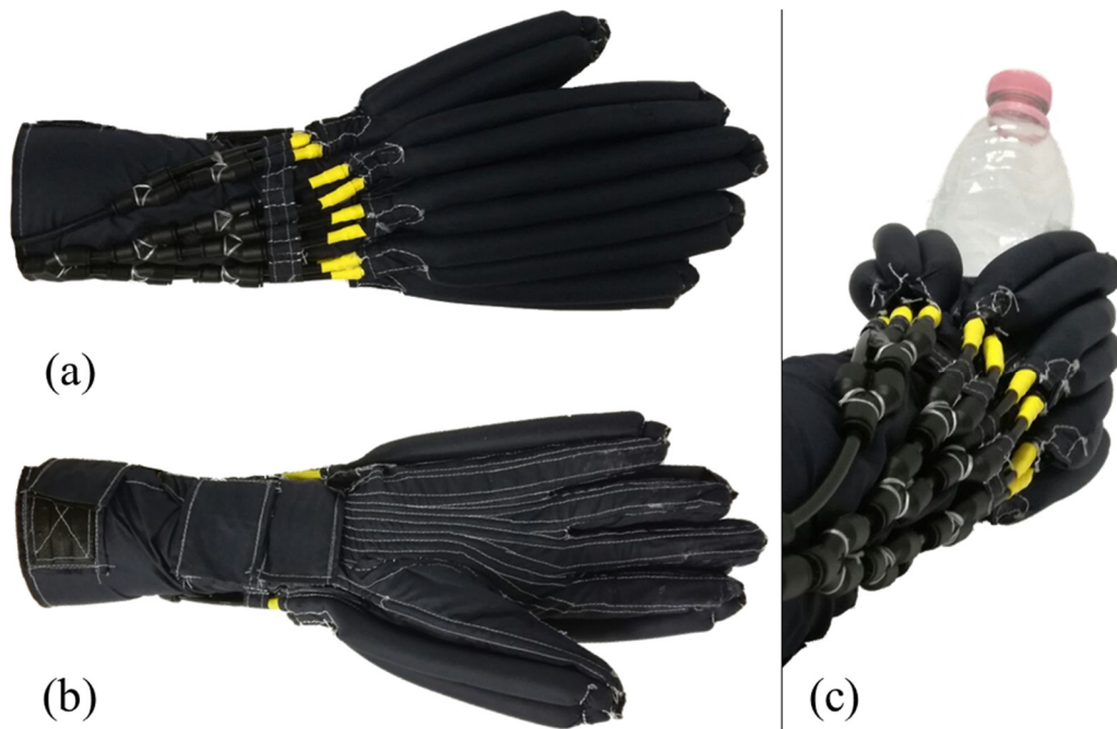
Figure 66 – Overview of the AirExGlove: (a) hand dorsal side of the system (pneumatic chambers pressurized), (b) hand palm side (tendon channel seams visible in white) and (c) side view of the system (thumb side) when grasping a plastic bottle.
