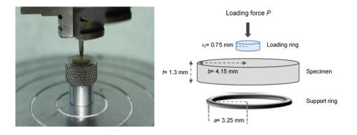
Figure 2-1 Biaxial flexural strength testing apparatus
