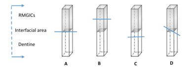
Figure 3-2 Mode of failure, A: adhesive failure, B: cohesive failure within the RMGICs, C: cohesive failure within the dentine, D: mixed failures
