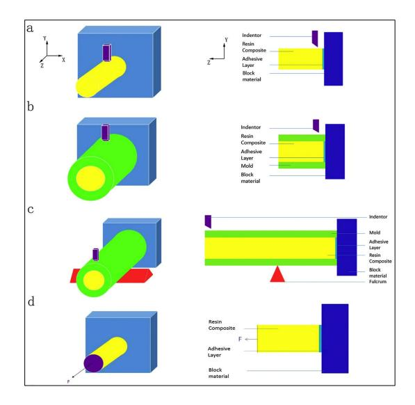
Figure 1-11 The schematic picture of (a) SBS test, (b) MESBS test, (c) LIME-SBS test, (d) TBS test, (Taken from Jin et al., 2016)
