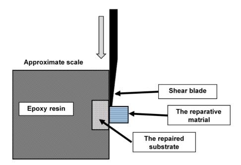
Figure 5-2 Diagrammatic representation of shear jig apparatus and shear force applied
