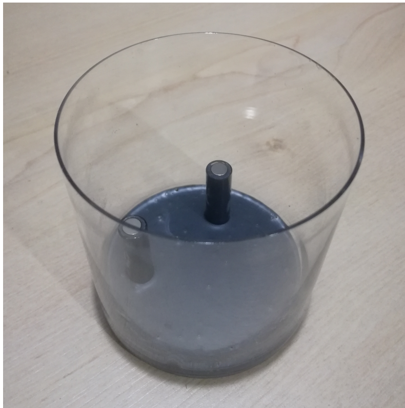
Figure A.2: The tank, showing pillars used to hold slides and fish in the centre
