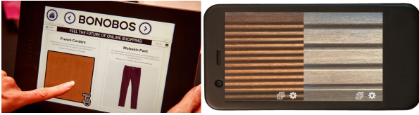
Fig. 2: Example applications which allow users to experience selected surface properties of offered products on websites using surface haptics displays (left: Tanvas Touch tablet [21], right: TPad Phone [22]).
