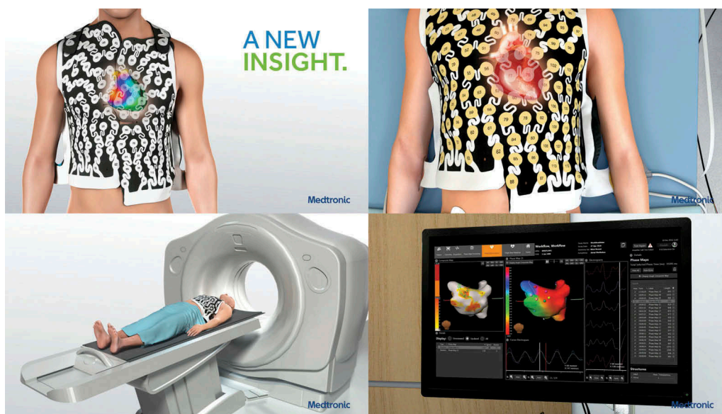
Figure 1. The 252-lead vest records torso surface electrograms. Reproduced with permission from MEDTRONIC.
