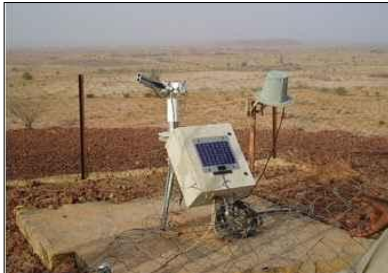
Figure 1.8 Sun-Photometer Ground station at Banizoumbou to measure the (AOT) of the atmospheric aerosol. (Source: http://aeronet.gsfc.nasa.gov/ )
