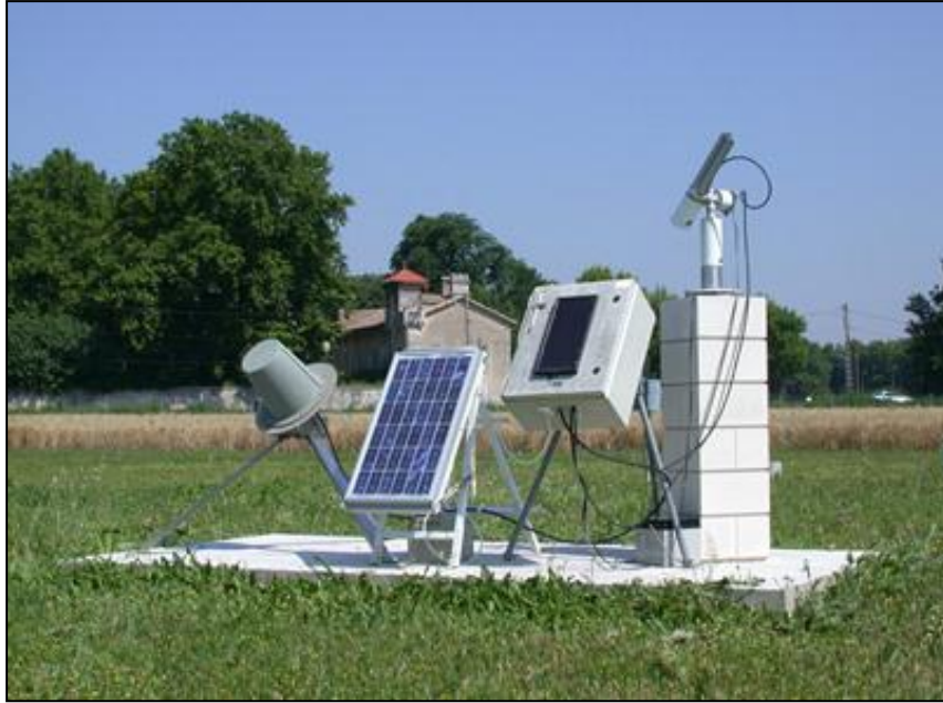
Figure 1.6 Sun-Photometer Ground station, one of the 29 ground stations distributed over Sahara to measure the (AOT) of the atmospheric aerosol. (Source: http://aeronet.gsfc.nasa.gov/ )
