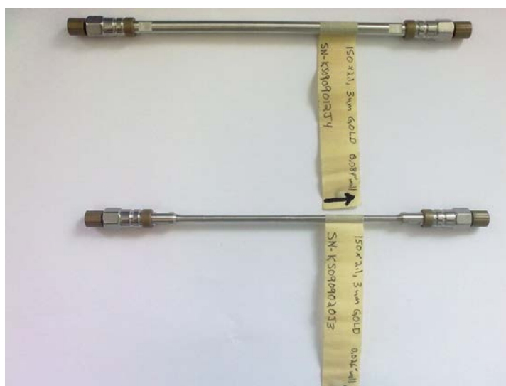
Figure 3.4. (Top) Standard 0.084" Thermo column hardware and (Bottom) modified 0.026" hardware.
