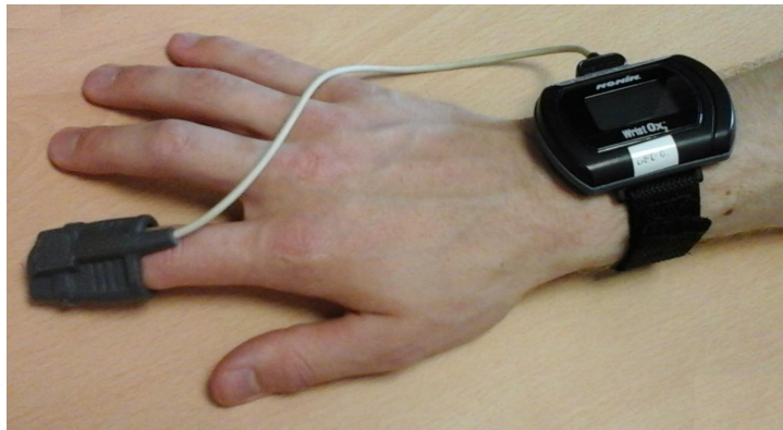
FIGURE 2.1: A wrist-worn wearable sensor: Nonin Medical's WristOx 2 ® 3150 measures heart rate (HR), arterial blood oxygen saturation (SpO 2 ), and the photoplethysmogram (PPG) continuously. Source: [5] (CC BY 4.0, DOI: 10.5281/zenodo.166546 )
