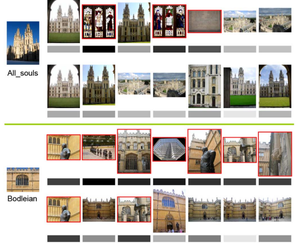
Fig. 2. Illustration of the top-ranked retrieval results for two queries on Oxford dataset. The two rows of search results correspond to the initial TFIDF scoring and D-sim re-ranking results. Each grey square beneath the image represents its distinctiveness weight in the context of brightness. False alarms are marked with red boxes.
