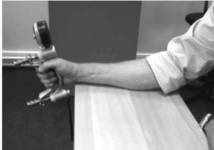
Figure 3.8 Hand grip strength testing using a hand grip dynamometer
