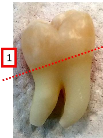
Figure 11 – Creation of enamel specimens was conducted using a cutting machine to section teeth in 3 places to produce the enamel slabs (Labcut 1010, Agar Scientific Limited, UK)
