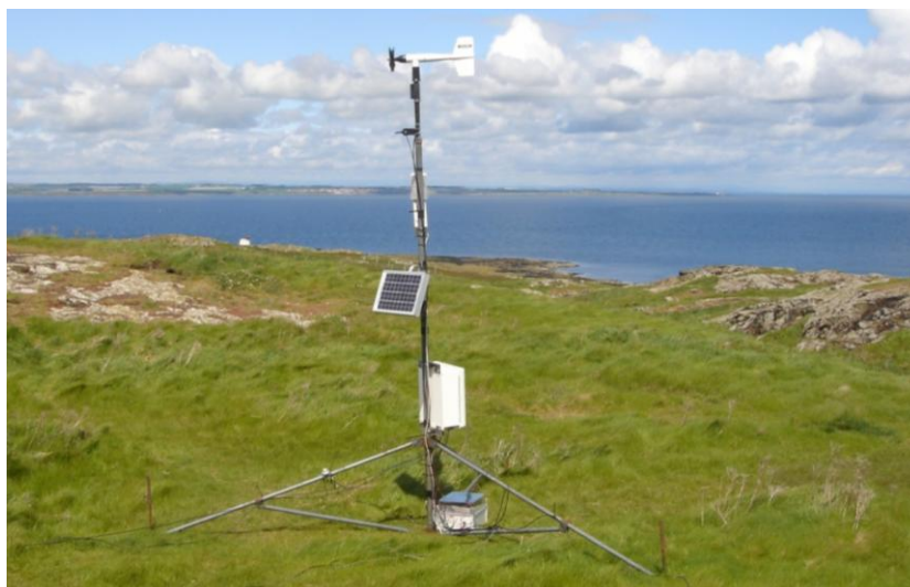
Figure 5.19 Weather station in-situ on the Isle of May, collecting data on temperature, humidity, solar radiation, rainfall and ground temperature.
