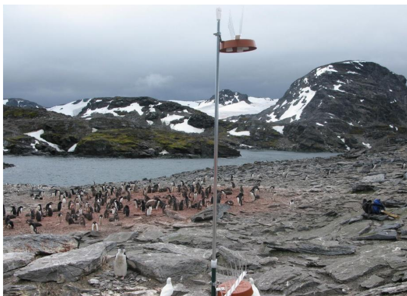
Figure 5.26 Mast 1 (with triplicate ALPHA samplers at three heights) looking west on Gourlay Peninsula, Signy Island, during the penguin breeding season. Image courtesy of Dr. P. Hill, University of Bangor.
