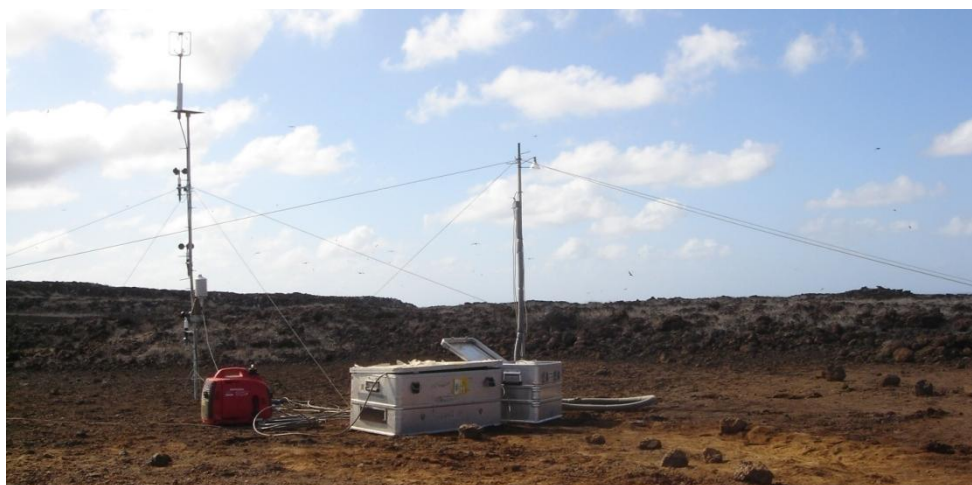
Figure 5.12 The set up of instruments used to measure the NH 3 concentrations actively from the Sooty Tern colony in Mars Bay. The AiRRmonia instrument was used to measure the NH 3 concentrations. The air inlet was positioned at 2 m above the ground. Instruments were powered by a Honda Eu10i petrol generator. Micrometeorological parameters were measured with a Gill Windmaster Pro sonic anemometer, on top of the mast 2.5m above the ground. Wind speed was recorded at three heights (2m, 1m and 0.5m) and the temperature, relative humidity and solar irradiance were measured at 0.75m above the ground.
