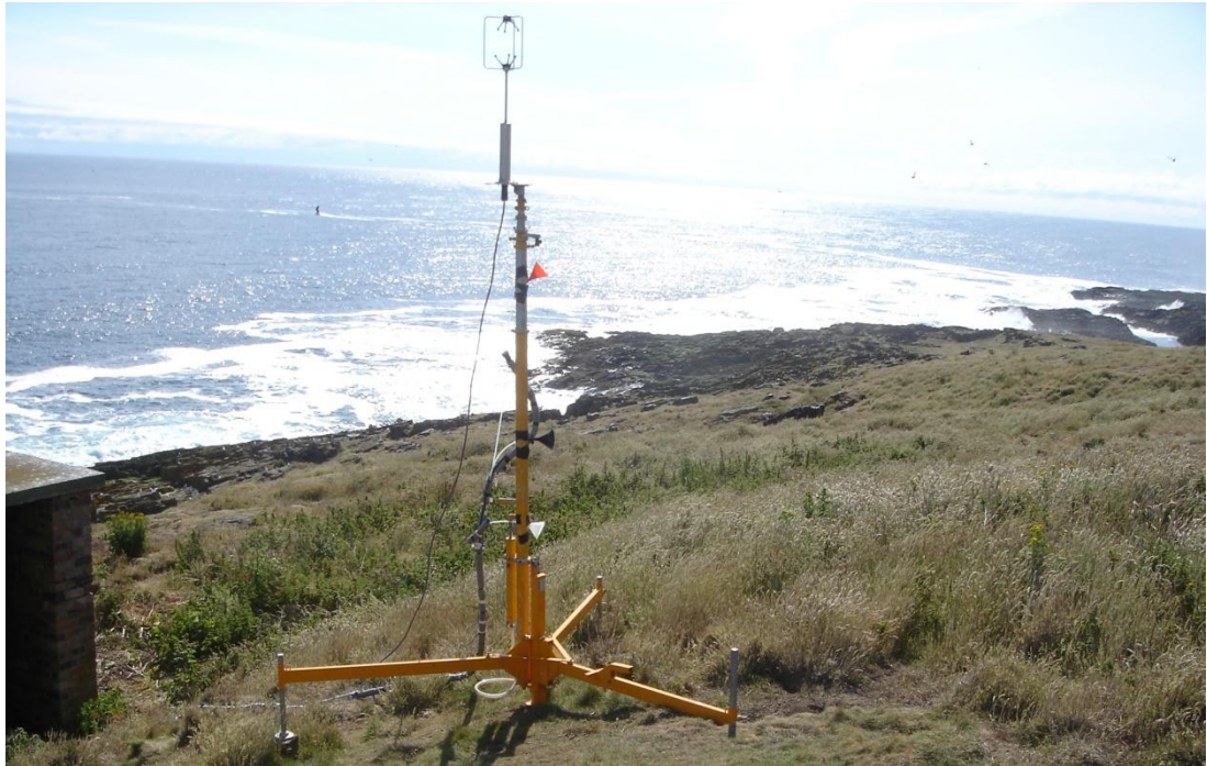
Figure 5.21 Sampling NH 3 concentrations and collecting turbulence data on the Isle of May, Summer 2009. The image shows sampling at three heights. Measurements were taken from the middle inlet (black funnel).
