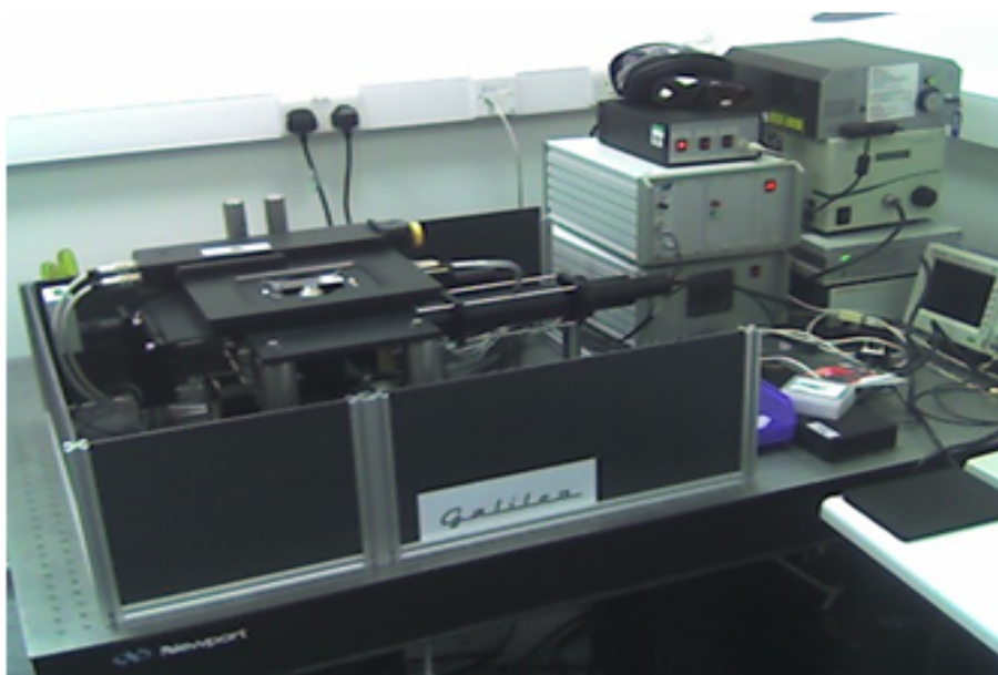
Figure 1.3: The ‘Galileo’ time-domain FLIM microscope at King’s College London: Pictured is an in-house developed time-domain FLIM system at the Randall Division of Cell & Molecular Biophysics, King’s College London. Details of the design, the various components, development, and some of the research that has been carried out using ‘Galileo’ and other similar in-house developed systems are presented in [62] and on our group website ( http://users.ox.ac.uk/~atdgroup ).
