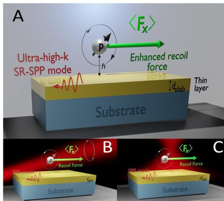
FIG. 1. Schematic diagram of a circular electric dipole above a thin metallic slab. Two possible experimental realizations are shown: b) a polarized plane wave illuminating a Rayleigh particle at grazing angle to the surface and c) a linearly polarized Gaussian beam at normal incidence focused near a particle, which is located away from the beam's axis.
