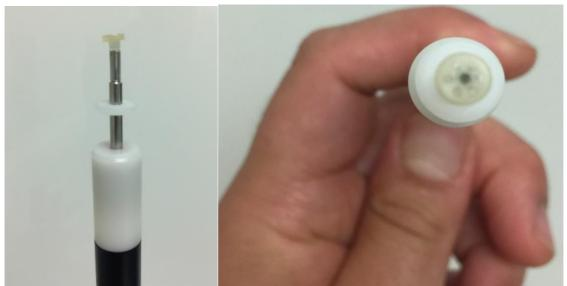
Figure 2-9 Close-up photo of pneumatonography probe
