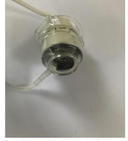
Figure 2. Close-up view of the coupling cone and transducer.
