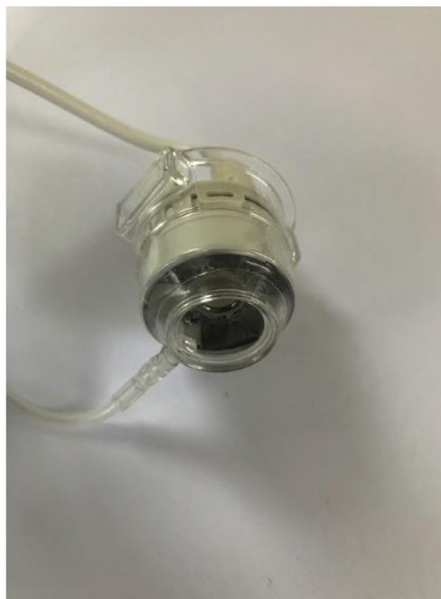
Figure 2. Close-up view of the coupling cone and transducer.
