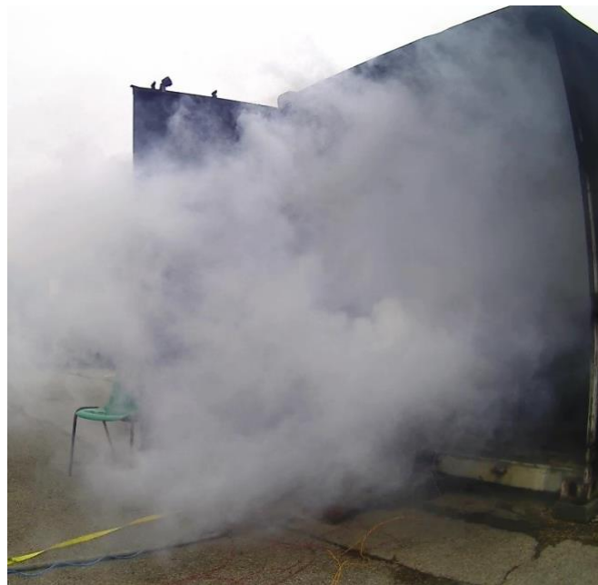
Figure 9. Stills from the video taken of experiment 2 at the Fire Services College: nail penetration at 50% SOC. Image (a) was taken 26.47 s after the nail penetrated the module completely; (b) was 35.47 s after penetration and (c) 52.13 s after penetration.
