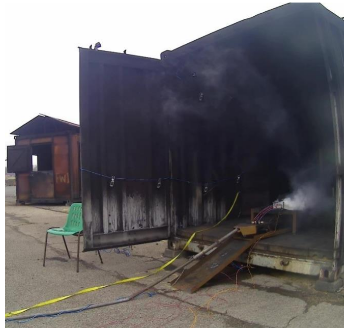
Figure 8. Images taken during experiment 1 at the FSC (nail penetration at 75% SOC): (a) 0.532s, (b) 0.538s, (c) 3.794s, (d) 3.858s, (e) 10.567s and (f) 82.6s after nail penetration.
