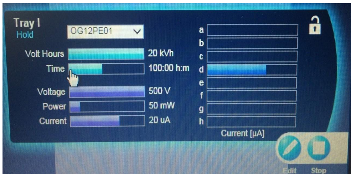
Figure 5: Isoelectric focussing run time information. Full separation over 20kVh completed in just over 18 hours.
