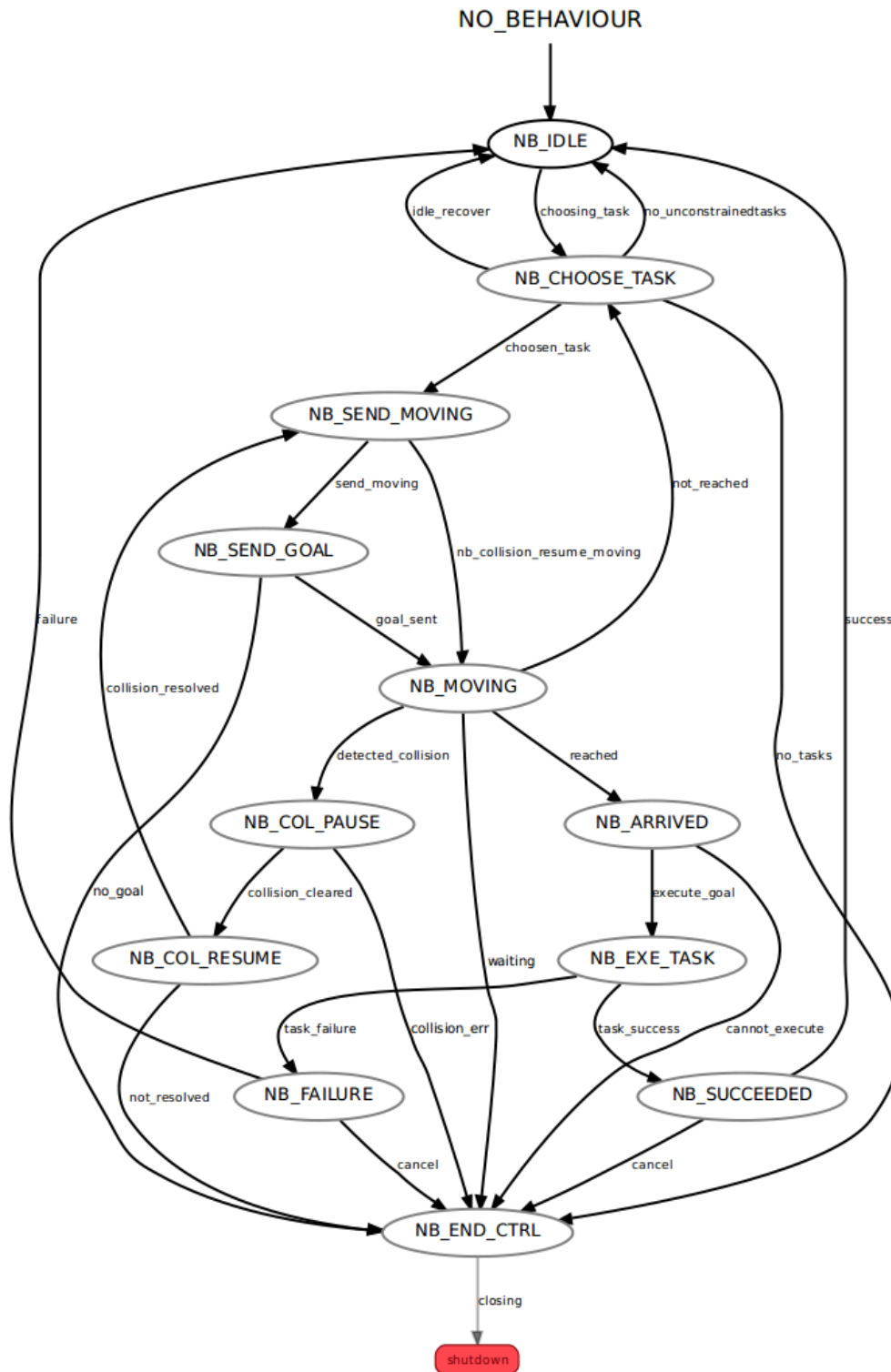
FIGURE A.2: Finite State Machine of a task executioner agent for NB.
