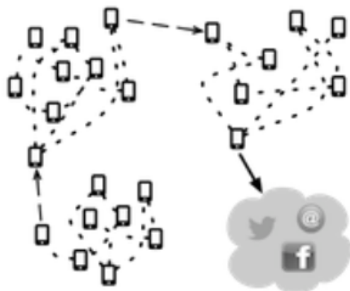
FIGURE 2.11: A diagram demonstrating how ad-hoc network based application connects offline client to an online server [85].
