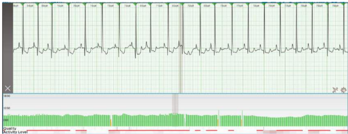
Figure 2.14. ECG recording (top) and tachogram (bottom). Each green bar in the bottom indicates an IBI measured on the ECG recording on the top. Shaded green bars represent artefacts that are automatically removed by Cardioscope™ ANALYTICS software from the measurements.
