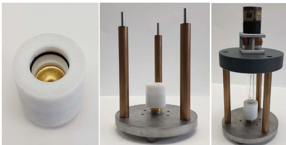
Electroplating cell set-up. Left: gold bullet sealed within PTFE holder; centre: bullet and holder mounted on the electroplating stand; right: with glass cell and platinum anode in place. The gold bullet serves as cathode.
