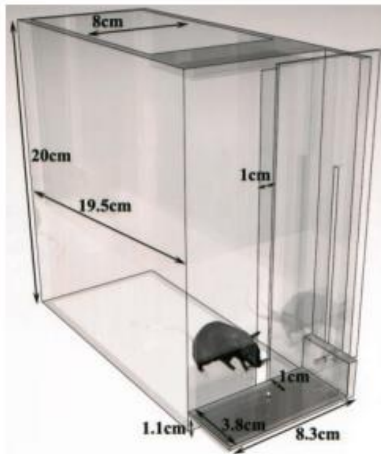
Figure 4 A single pellet reaching task for mice
