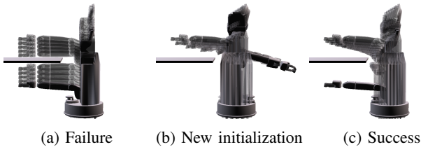
Fig. 4: Initialization-based explanation. An optimization-based planner uses straight-line initialization and fails to find a trajectory (a). It then finds initialization (b) which leads to a feasible plan (c). It provides Explanation 3.
