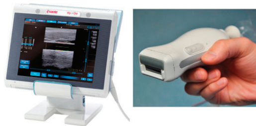
Figure 14. Portable imaging scanner combining photoacoustics and ultrasound. Left is the ultrasound scanner system and right is the picture of the probe integrating the laser module and ultrasound transducer array. Reprinted with permission from K. Daoudi, P.J. van den Berg, O. Rabot, A. Kohl, S. Tisserand, P. Brands, and W. Steenbergen, Optics Express , Vol.22, pp. 26365–26374, 2014; licensed under OSA’s “Copyright Transfer and Open Access Publishing Agreement” (OAPA). Copyright 2014 Optical Society of America.
