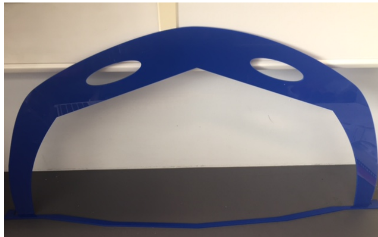
Figure 3.1: Laser cut plastic arch template of 3T scanner bore.
