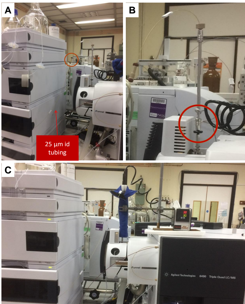
Figure 2.11 micro-flow LC-MS/MS set up; A) the connection of the micro-autosampler to the column was optimised to minimise dead volume by using PEEKsil tubing with internal diameter of 25 µm. An inline micro-filter was also used. B) A close-up photo of the unique column connection set up directly connected to the ESI course using a coupler. C) An overview over the instrument set up showing the column temperature control using a hot pocket set to 30 °C.
