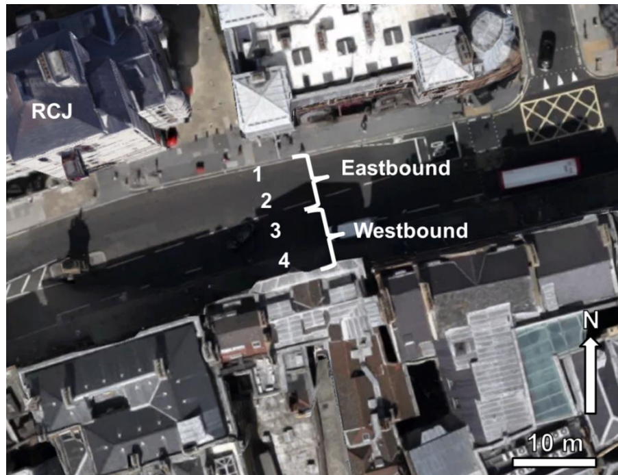
Figure 2.8: Approximate location of the traffic count site relative to the south east corner of the Royal Courts of Justice (RCJ). Lanes are number 1:4 with lanes 1 and 2 carrying eastbound traffic, and lanes 3 and 4 carrying westbound traffic. Lanes 1 and 4 are nearside (adjacent to the kerb) and lanes 2 and 3 are offside (non-adjacent to the kerb).
