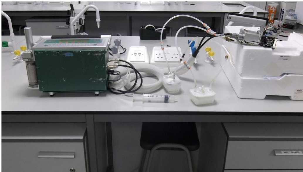
Figure 2.5: Equipment used for measurement of CO 2 fluxes from river water.
