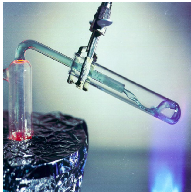
Figure 3-1: Images of novel nuclear fuel physical forms. Left – cross section of TRISO fuel, showing <1 mm kernels fissile material surrounded by layers of graphite and silicon carbide, dispersed within a graphite matrix [34]. Right – molten lithium beryllium salt of the type under consideration for use in many Molten Salt Reactor (MSR) designs [35].
