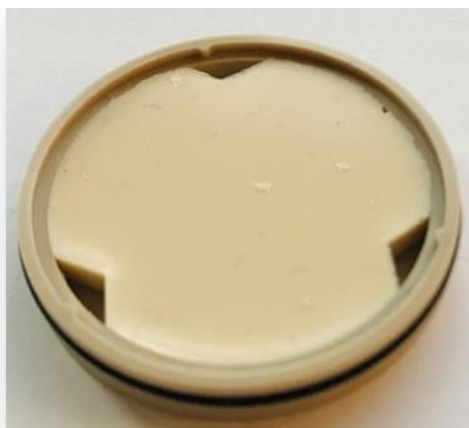
Figure 62. Photograph of the combined oxygen module. The skeleton (produced by CNC-drilling from PEEK) combined with an oxygen-generating disk and an O-ring.
