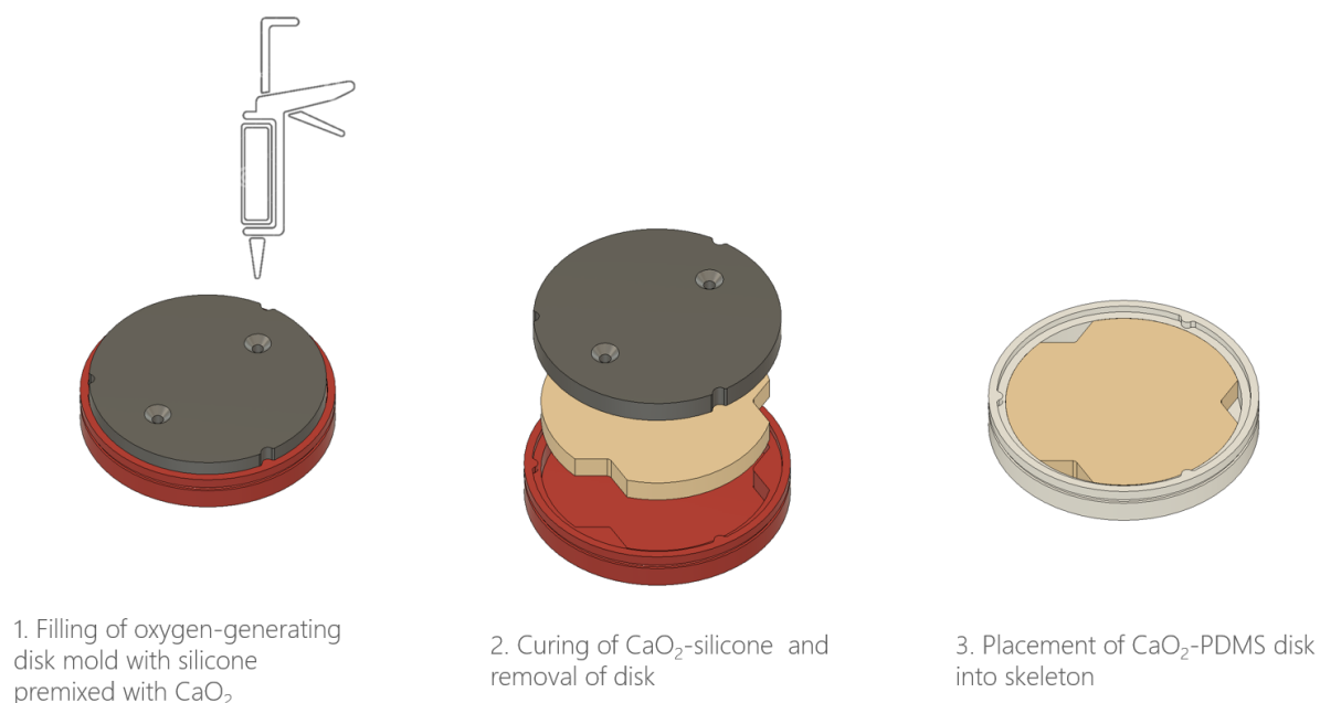
Figure 61. Production process of the oxygen module. The curing mould with triangular extrusions is filled with medical grade silicone premixed with \text{CaO}_2 . After curing of the silicone, the oxygen-generating disk is removed and placed in the skeleton of the encapsulation device.
