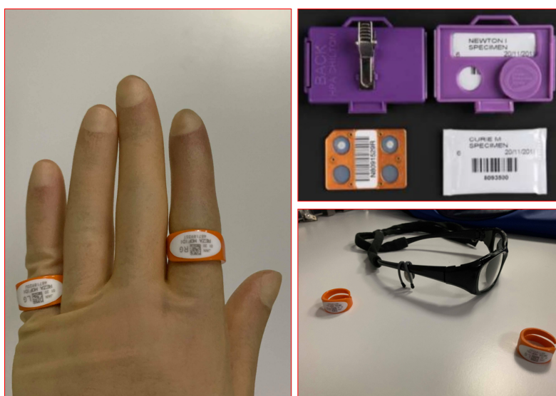
Figure 1.3 Examples of Thermo-luminescent Dosimeter (TLD) Badges (Adapted from Public Health England, Body Thermoluminescence Dosimeter, 2018)
