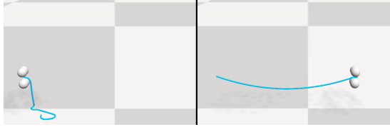
Fig. 4. Frames from the simulated environment. On the left – the beginning of the task where the cable falls freely; on the right – the gripper finished the task and holds the cable’s end.
