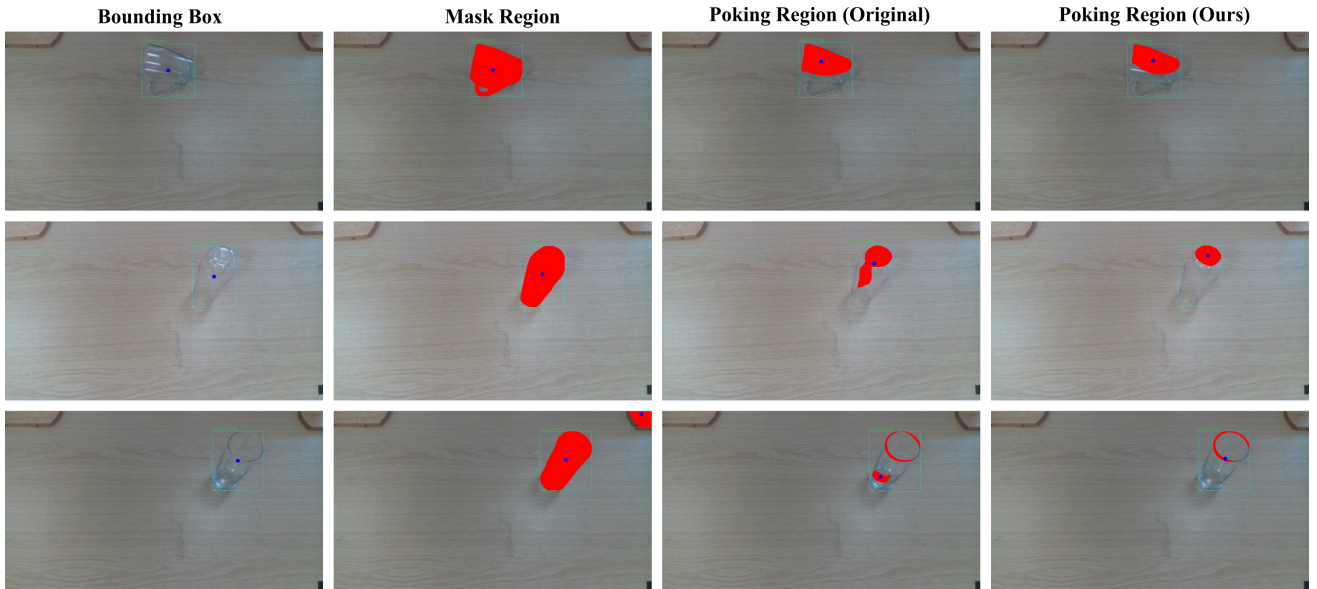
Fig. 8: Examples of the poking points generated with the bounding box, the instance mask, the poking region with vanilla Mask R-CNN loss (Original) and the poking region with our PN loss (Ours). The red colour and blue dot represent the segmentation results and generated poking points, respectively.
