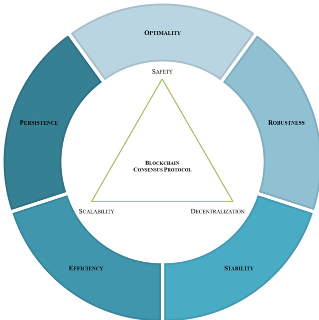
Fig. 6. Visual representation of the Blockchain Trilemma in relation to the PREStO framework. The tradeoff between Safety, Scalability, and Decentralization is precisely captured by the corresponding subcategories in optimality, efficiency, and stability. Robustness and persistence offer alternative approaches for a long-term resolution of the Trilemma.
