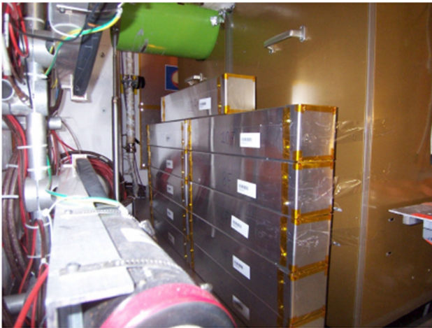
Fig. 5 A photograph of the prototype MMT detector deployed at IP8
