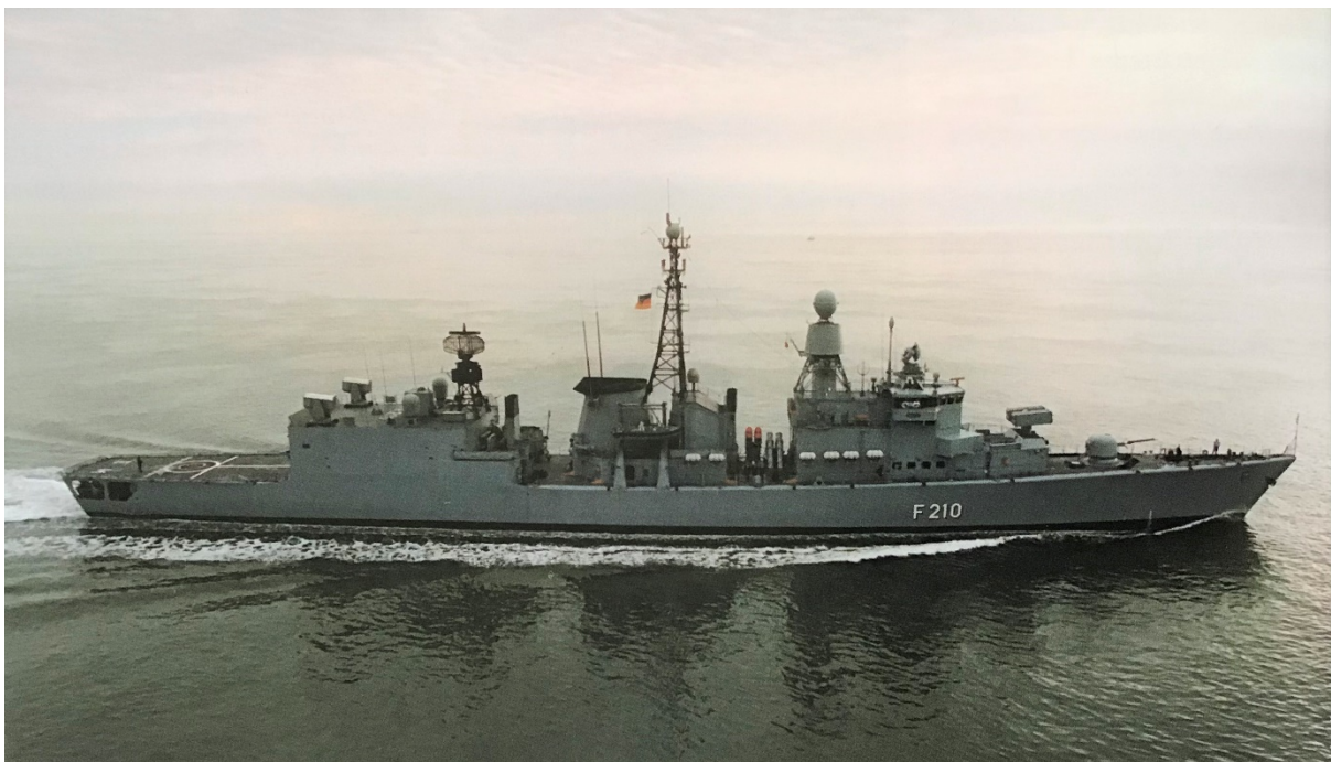
Fig. 42, Type 122 frigate Emden, ending Sharp Guard on 21 st July 1996, speedboat instead of cutter, 20mm gun just aft of the bridge-wing (Source: Ingo Wagner, picture alliance)
