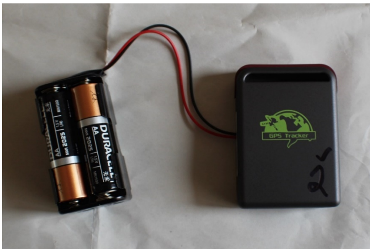
Appendix figure 1 GPS tracker with battery retrofit.
