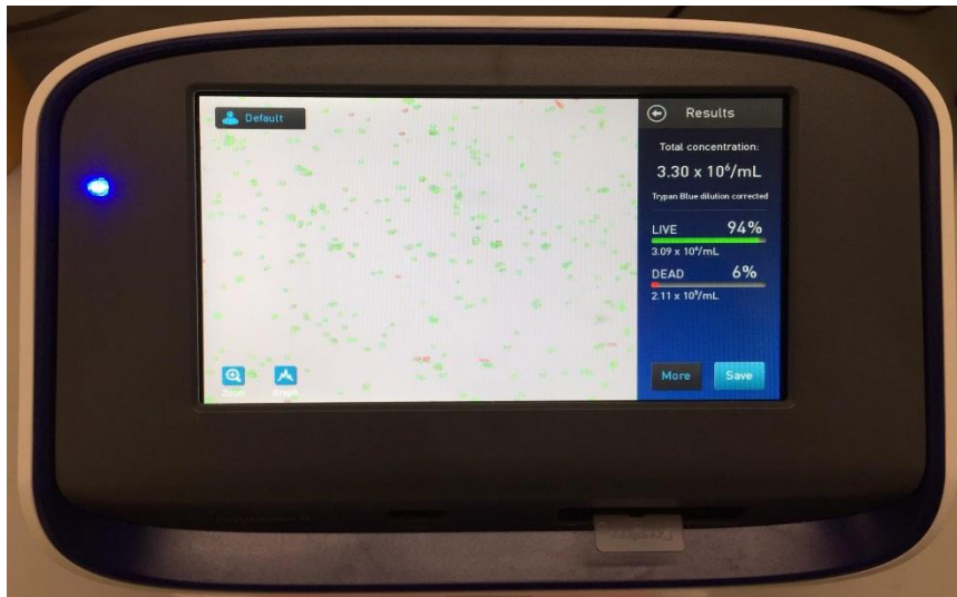
Figure 6. Trypan blue exclusion test for HepG2 cell using Countess® Automated Cell Counter
