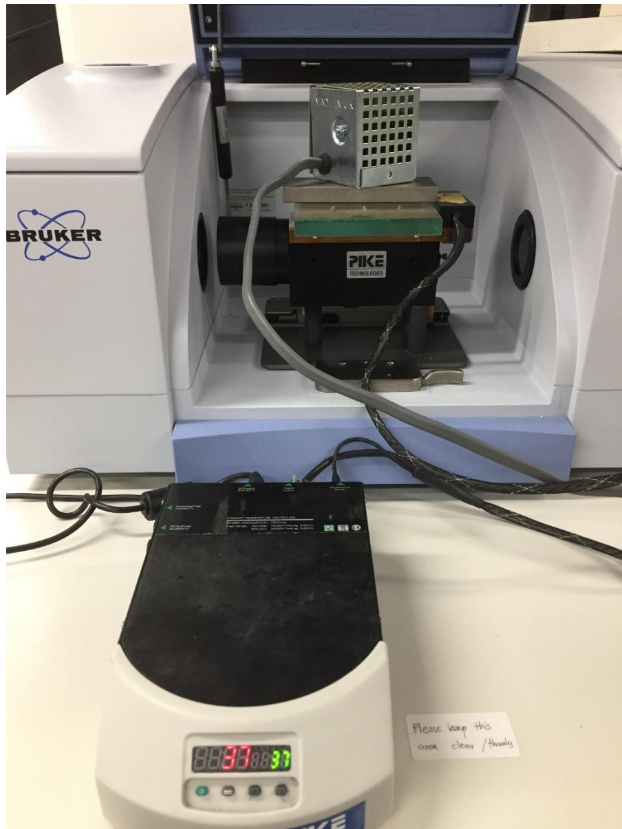
Figure 9. Photo of Bruker spectrometer modified to a temperature-controlled ATR plate for the live-cell FTIR measurement
