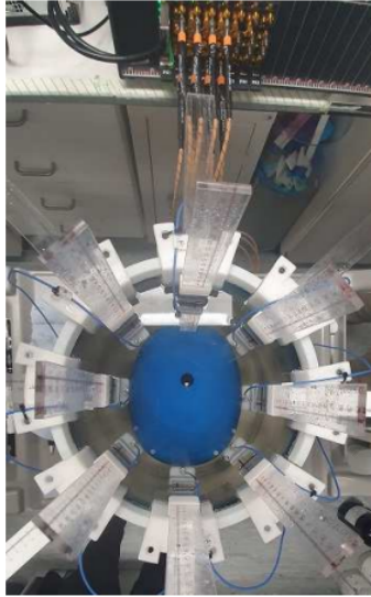
Figure 3.14: Measurement hardware and setup.
