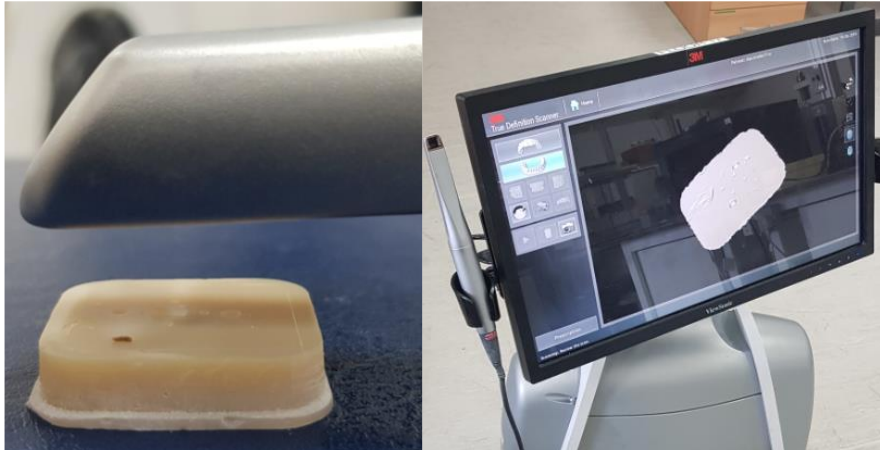
Figure 2-7 – Handheld scanning of the enamel sample and 3D data produced on the computer screen of IOS-TD.
