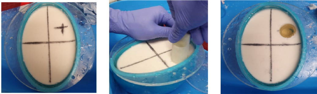
FIGURE 3.22: Elliptical brain phantom before (left) and after (right) inserting the eccentric target. The target was positioned at two different locations in the two constructed phantoms.
