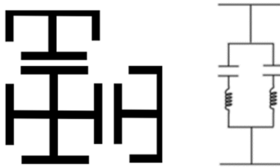
FIGURE 3.5: Jerusalem cross equivalent circuit.
