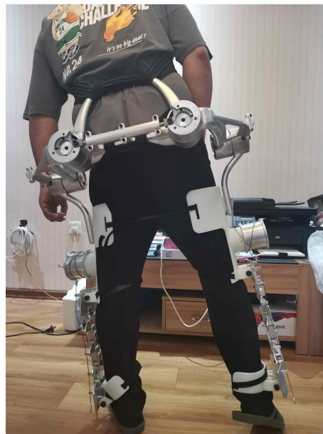
Fig. 10.16 Abdduction-adduction Movement of the Hip Joint
