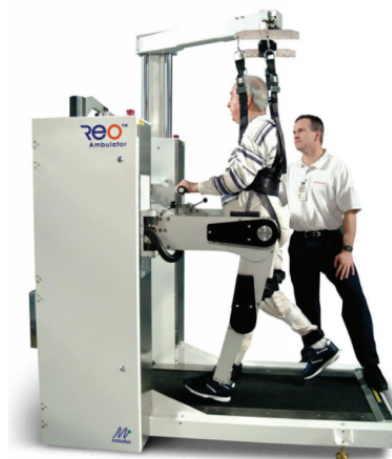
Fig. 3.20 ReoAmbulator Rehabilitation System [290]
