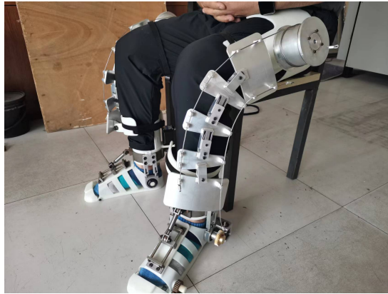
Fig. 10.7 The Bending State
