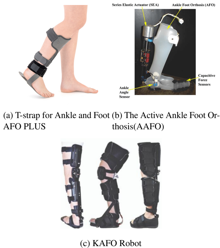
Fig. 3.6 Stationary Ankle Rehabilitation Robots [135, 52, 28]
