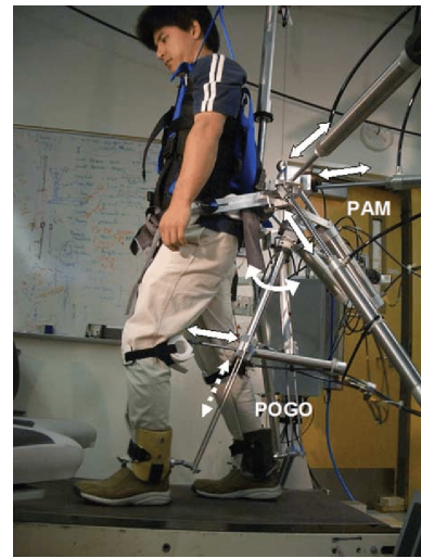
Sys-Fig. 3.12 The PAM and POGO Mechanism [254]
