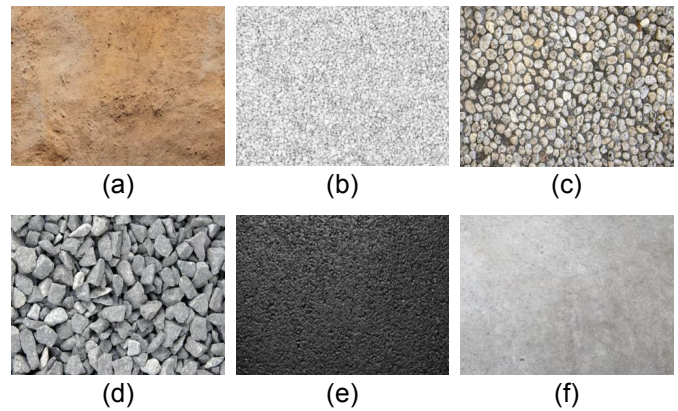
Fig. 1. Images of various types of roads based on the materials used for road surfacing: (a) Earthen road, (b) Gravel road, (c) Kankar road, (d) WBM road, (e) Asphalt road, and (f) Concrete road.
