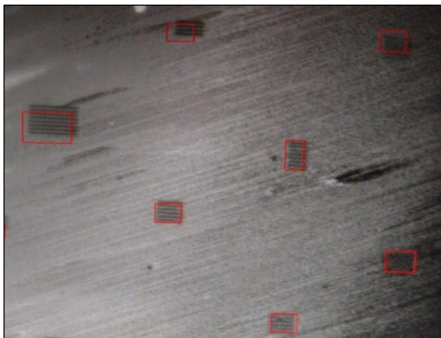
Figure 42: Representation of scanned areas by the laser. A glass slide covered with a fluorescent dye with seven red boxes of various sizes representing the different photobleached areas with the laser in a single acquisition. The pulse energy used is 100% for exaggerated and visualisation purposes.
