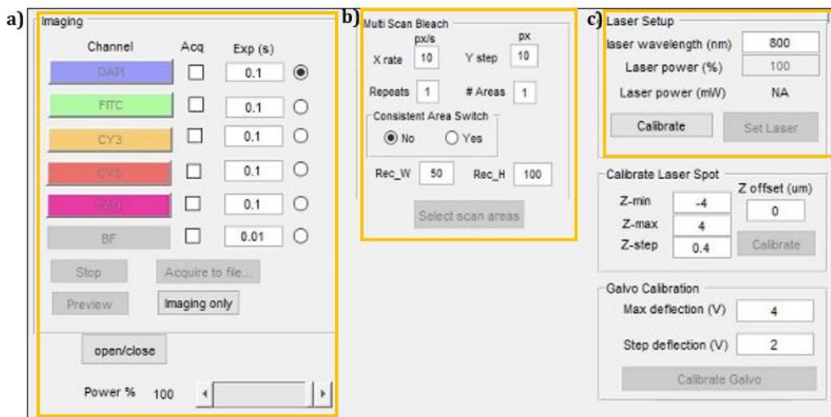
Figure 40: MATLAB user interface. Numerous parameters controlled via the in-house developed programme. The main parameters were a) the Imaging section, that controlled the selection of the fluorescent light, the exposure time and light intensity for image acquisition, b) the Multi Scan bleach, that controlled the laser wavelength and pulse energy and c) the Laser Setup, that controlled the horizontal scanning speed (x-rate), the vertical scanning step (y-step) and the number and size of the areas to scan.
