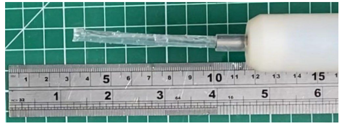
Fig. 8: Eversion of an 7 cm growing robot manufactured using the CO_2 laser welding method, everting with the actuation system of [13].
