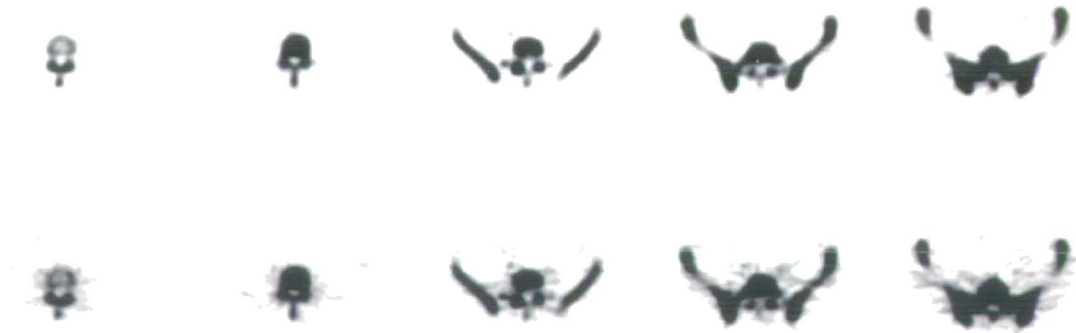
Figure 7.8. Heavily smoothed selected image planes from adult ^{18}\text{F} -F ^- pelvis study. Top: 3D mode. Bottom: 2D mode. From left to right: image planes 11,16,21,26,31. A 3-D Gaussian smoothing kernel of FWHM 7.5 mm has been applied to both image volumes, and the inverse grey-scale maximum has been set to 35% of the image maximum.
