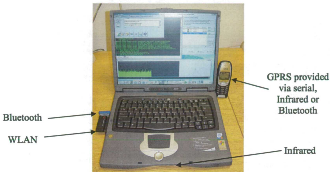
Figure 2-1: Interface heterogeneity. Clockwise from top-left, the picture shows a USB Bluetooth device, a WaveLAN PCMCIA Lucent card interface, an infrared interface and a GPRS enabled cellular phone connected to the laptop via serial, infrared or Bluetooth connection
