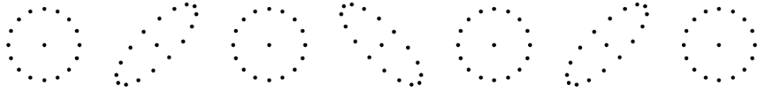
(b) The evolution of the \times mode gravitational wave. Time moves from left to right in the figure, and the circle's deformation oscillates like a \times sign [149].
