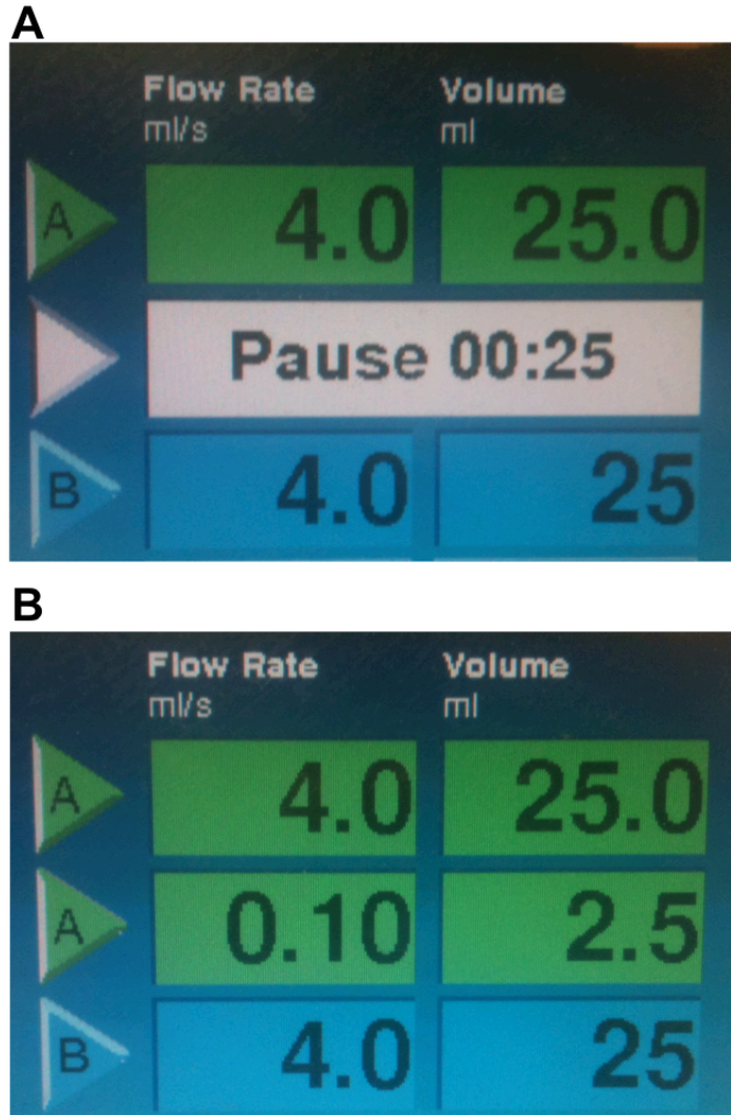
Figure 4.3 Programmed injector control in the case of the dual-head power injector with (A) and without (B) a “pause” function. Please see the text for details.
