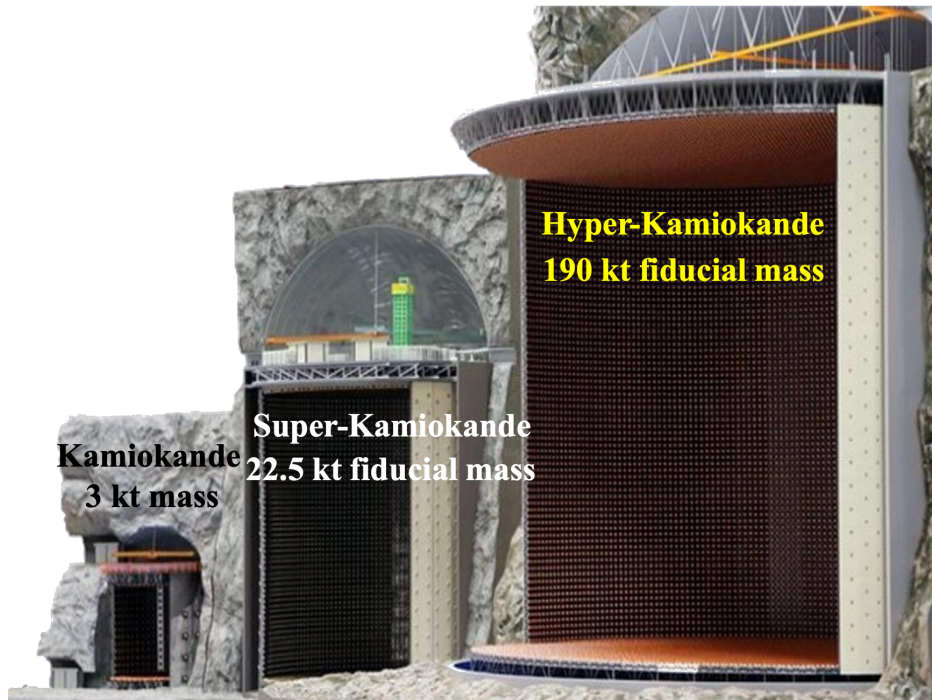
Figure 2.3: The size comparison of three generations of Japanese neutrino detectors [47]. The fiducial mass refers to the region in the inner detector where the neutrino interactions are analysed. This volume is placed to avoid regions near detector walls where background events due to cosmic rays or radioactivity can mimic or obscure genuine neutrino interactions.
