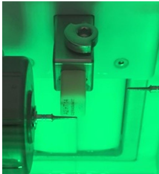
Figure 5-4 Block milled to manufacture the nano-resin ceramic antagonists
