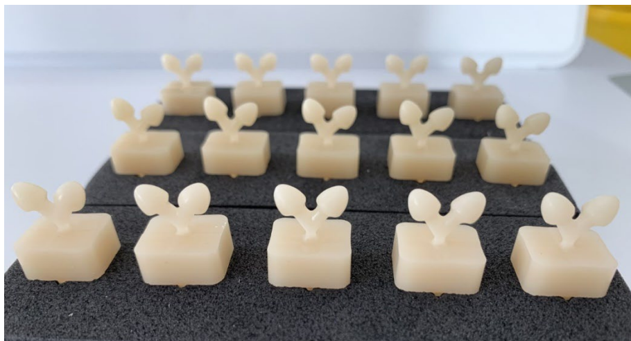
Figure 5-5 The milled-out antagonists - two per block which were separated after milling.
